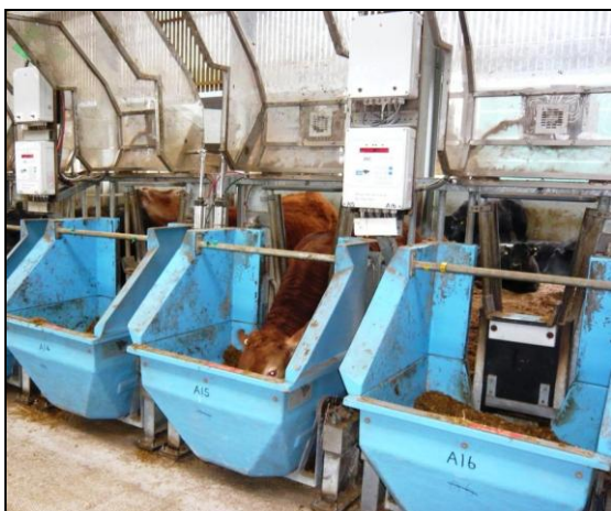
'Hoods' (opened for photo) used to measure methane emissions whilst livestock are feeding
