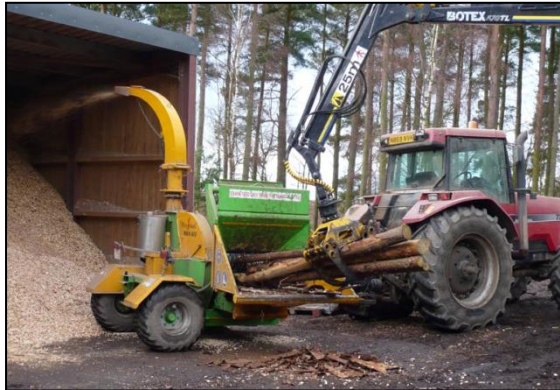
Chipper in action at the Estate sawmill
