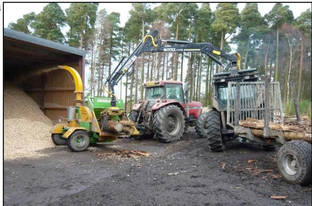
The Estate spent £28k on a chipper specifically for producing the right size of chips for the boiler. Again on the farm scale, farmers would be able to hire in these machines and do most of chipping over a day; key here would be making sure wood has been dried sufficiently and that there was enough space for storage for the chipped wood. At a suitable site, a chipper could blow chips straight into a storage area.
