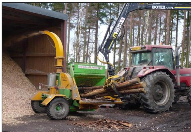
When considering a woodchip system, Peter noted that it was key to consider delivery and storage of the chip once on site; how will the system will work for your farm? At Floors, the chip is tipped into storage bays and then the hopper loaded using a telehandler. The Castle and Garden Centre use around 450 tonnes of chip per year; this is in contrast to around 40/50 tonnes that would be needed to heat a decent sized farmhouse. Chip sells at about £100/tonne.
